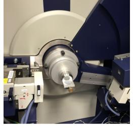
**Bragg-Brentano Diffractometer** Samples were measuerd with the Rigaku Ultima 4 from 5- 25 ° 2Theta for 0.5 min/° with 0.02° stepwith.
