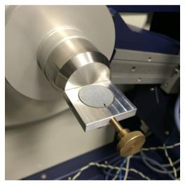
**New Sample Holder** New developed cylinder sample holder for x-ray diffraction analyses of UHPC cylinders.
